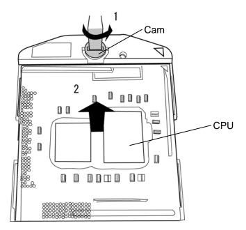
Figure 4-33 Removing the CPU
